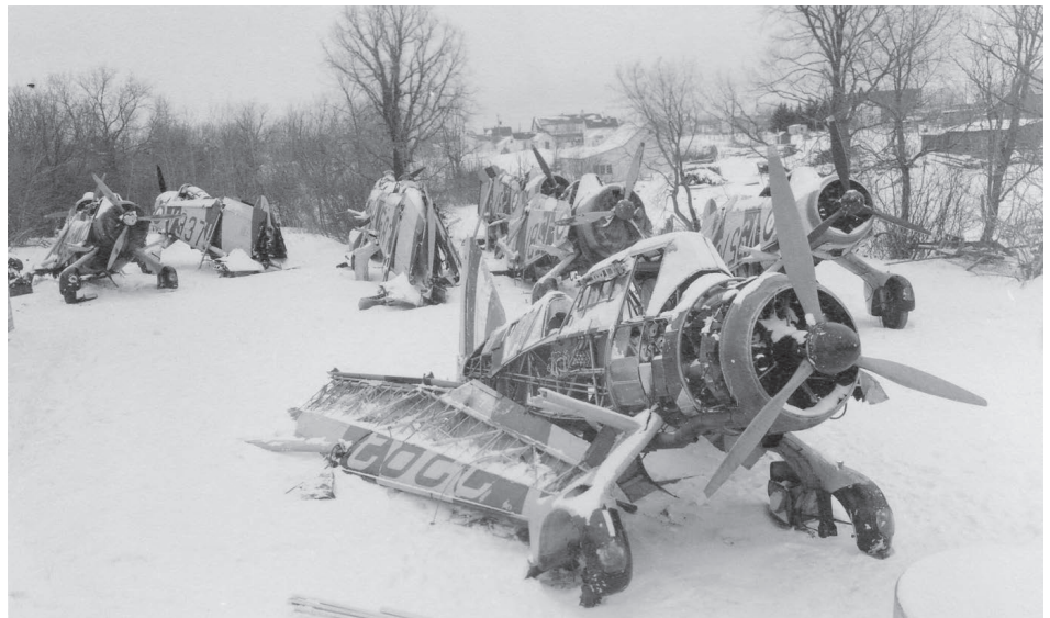
Brandt purchased surplus Lysander aircraft that were no longer needed by the Canadian government after the Second World War ended. The planes were specially designed to pick up and drop off spies behind enemy lines. The aircraft engines were made of aluminum, and were melted down in the Brandt foundry to cast and machine a variety of parts and components for other companies (MAID MHC 720-04).
